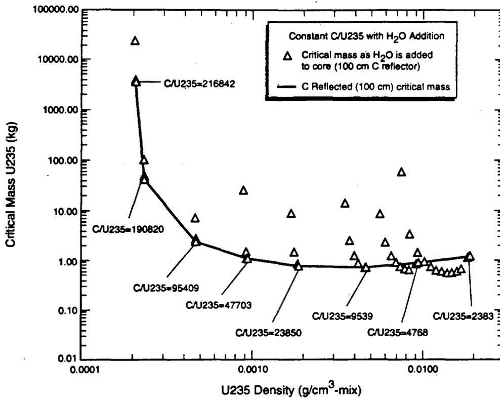
Figure 5.5 Critical mass of graphite-reflected U(93.2)C spheres as a function of H<sub>2</sub>O addition to the core.
