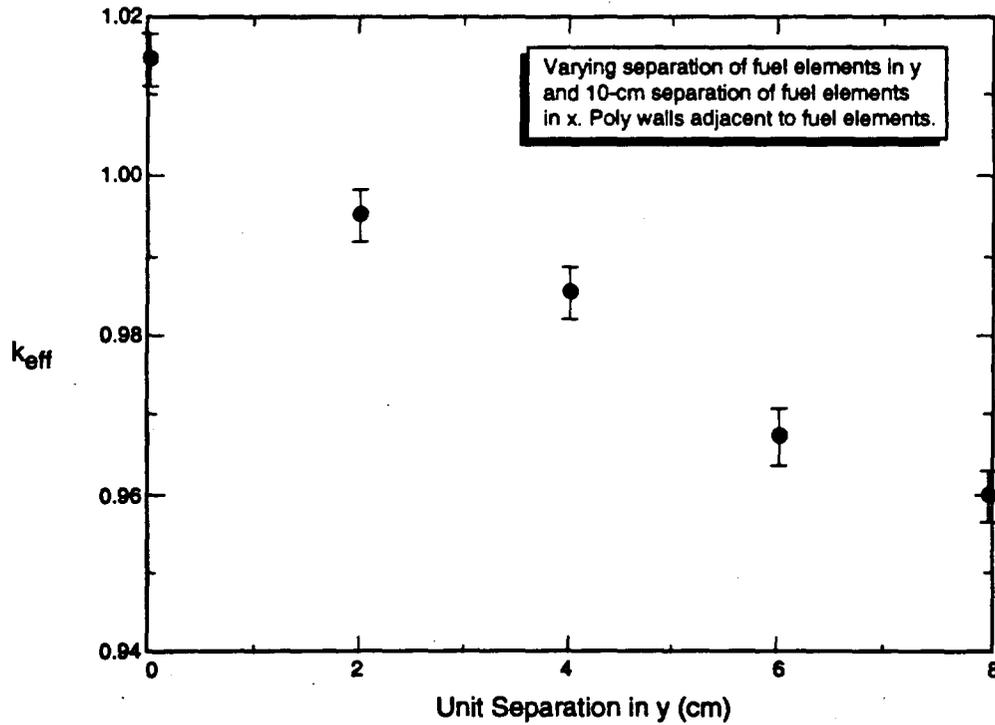
Figure 2.8.  $k_{eff}$ , with fuel elements fixed at 10cm separation in "x," as a function of separation in "y."
