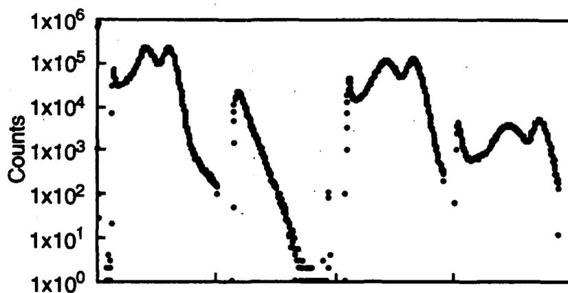
A quick run was made with a chamber centered outside of Big Ten rather than on an axis inside of Big Ten. A comparison of spectra inside and outside the assembly appears in Fig. 2.12. Note the dramatic change in relative fissions, attributable to room return of neutrons.
