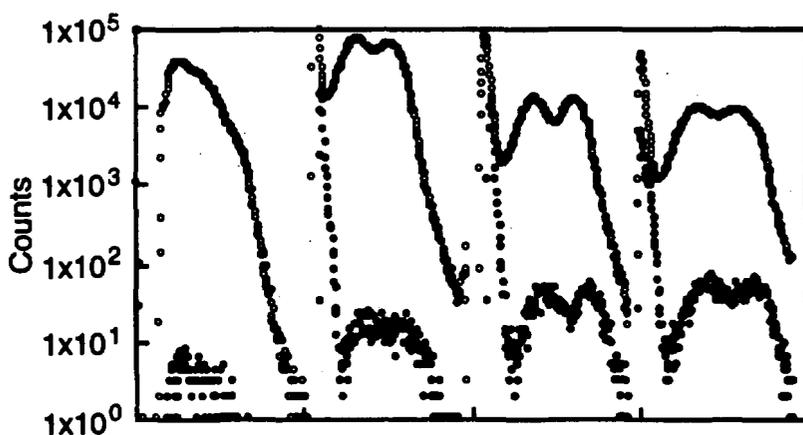
Figure 2.12. Comparison of spectra for a fission chamber inside of Big Ten (open circles) and outside of Big Ten. Note the change in relative intensities.
