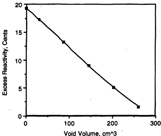
Figure 2.13. Total excess reactivity as a function of void size in Big Ten.
