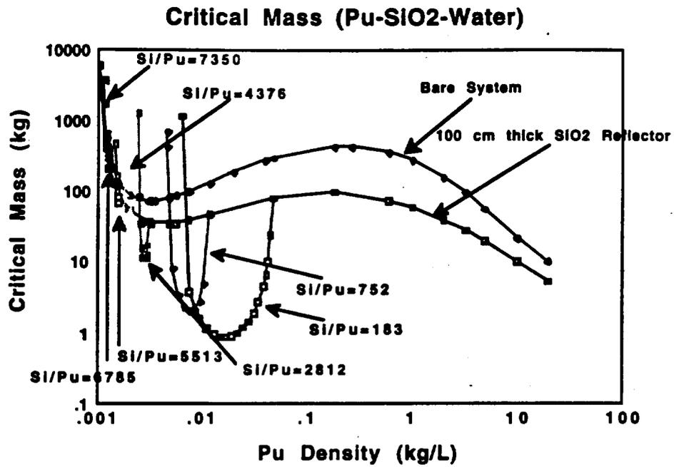
Figure 5.3. Critical masses of SiO<sub>2</sub>-water-moderated Pu spheres.
