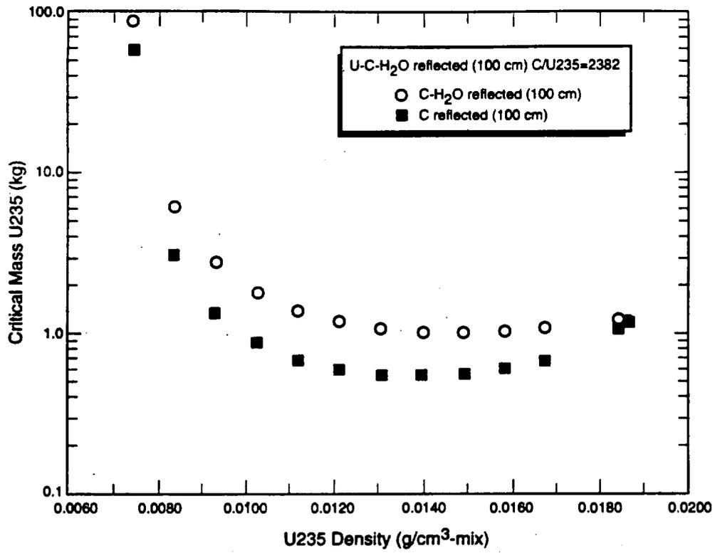
Figure 5.7. Critical mass of graphite-reflected and graphite-water-reflected U(93.2)C spheres as a function of H<sub>2</sub>O addition to the core.
