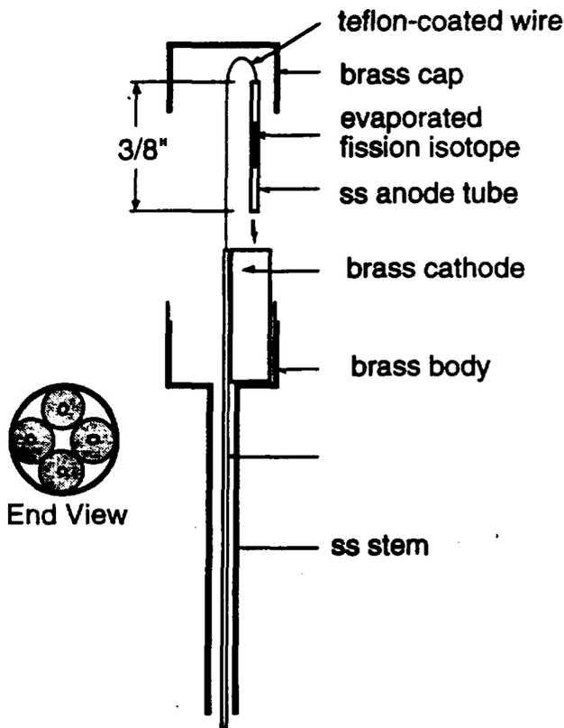
Figure 2.10. Design of the four-barrel fission chamber.
