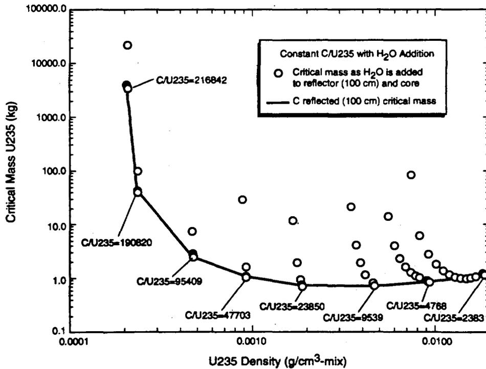
Figure 5.6. Critical mass of graphite-water-reflected U(93.2)C spheres as a function of H<sub>2</sub>O addition to the core.
